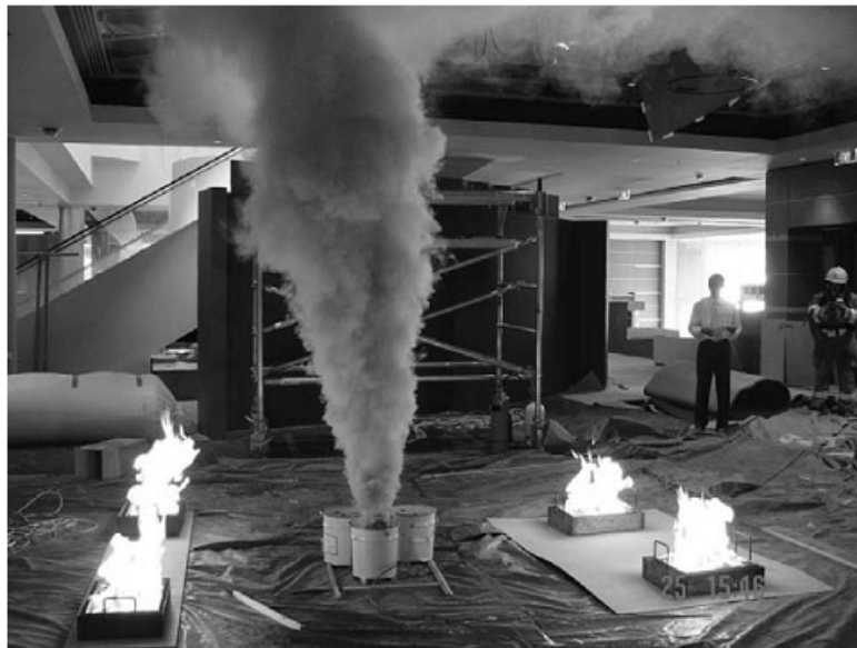
Fig. 1. Typical hot-smoke test layout using smoke canister [15].
