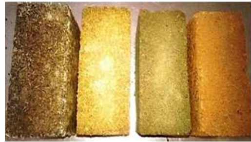
Figure 7. From left to right: Cement+roast wood fibre composite; Composite of cement+rice husks; Agglomerate; Composite of cement+bar soil (O. Godonou, 2015).
