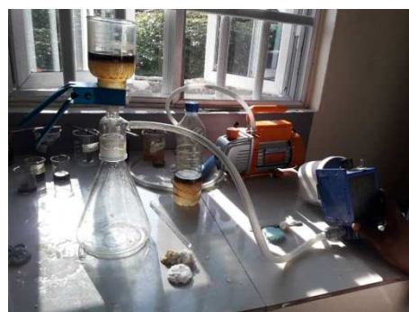
Figure 2. Membrane Separation Process using vacuum pump.
