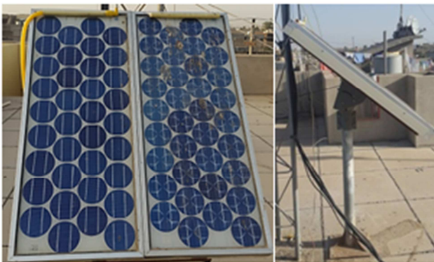
Fig. 1. Installation of PV test modules on the base.
