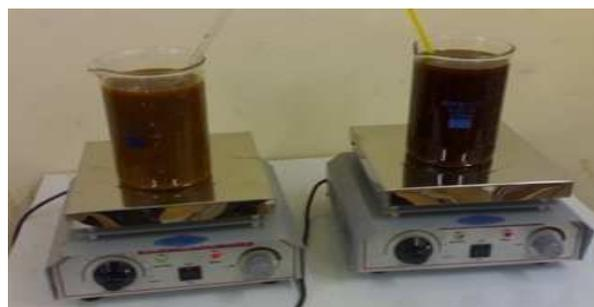
**Figure 2.1.** Experimental set up during degumming process for purification of crude castor oil
