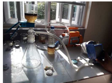
Figure 2. Membrane Separation Process using vacuum pump.
