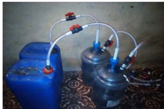
Figure 3. Biogas Digestion plant.
