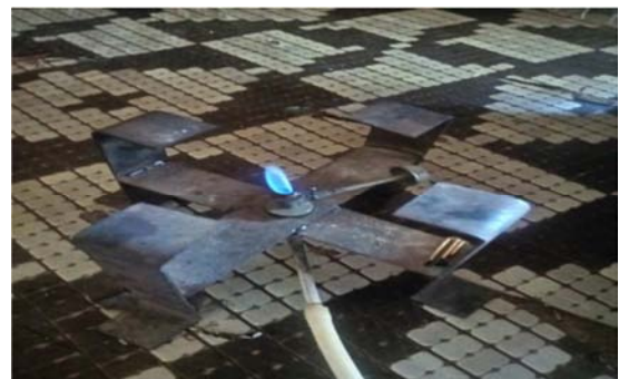
Figure 8. Constructed Burner showing clear blue flame of the biogas produced.
